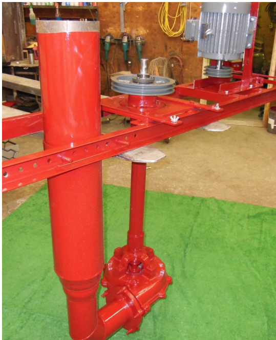
Pump with Motor and Sheaves on the mounting base ready for
